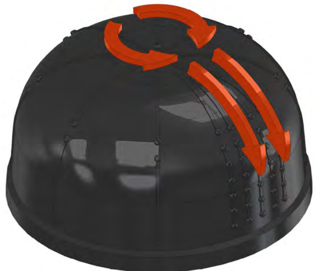
Zilmet Diaphragm – 3D Model Showing Side Connection Flow Dynamics
